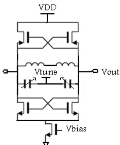
Fig. 1. LC- VCO circuit diagram.
