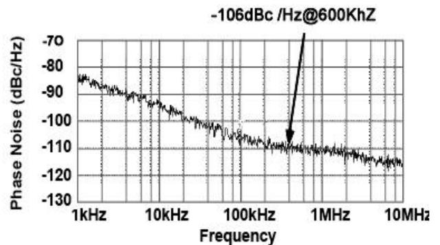
Fig. 4. The measured phase noise against offset frequency.
