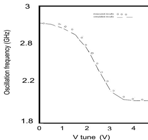
Fig. 6. The Simulated oscillation frequency against offset voltage.
