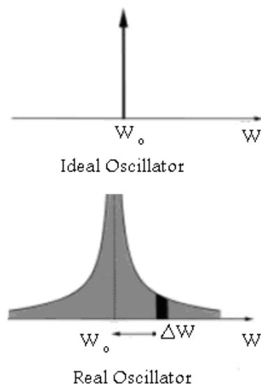
Fig. 2. Illustration of phase noise in frequency domain.
