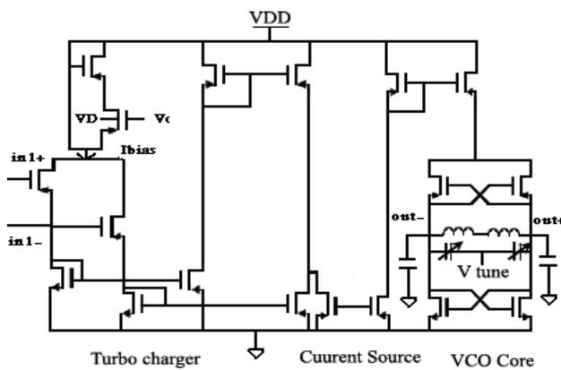
Fig. 3. Core circuit prototype for LC VCO.
