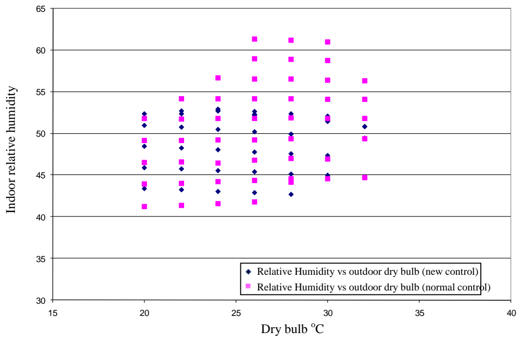
Fig. 8. Comparison of indoor relative humidity vs. outdoor dry bulb in new and conventional control for AHU-8 (0.4% dry bulb temperature design condition).
