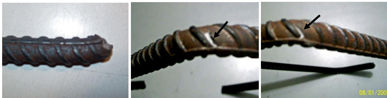
Fig. 14. Cracks and fracture of steel bars during bending on site [provider 'T'].
