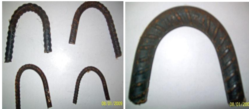
Fig. 9. The acceptance of steel bars based on the results of cold-bend tests.
