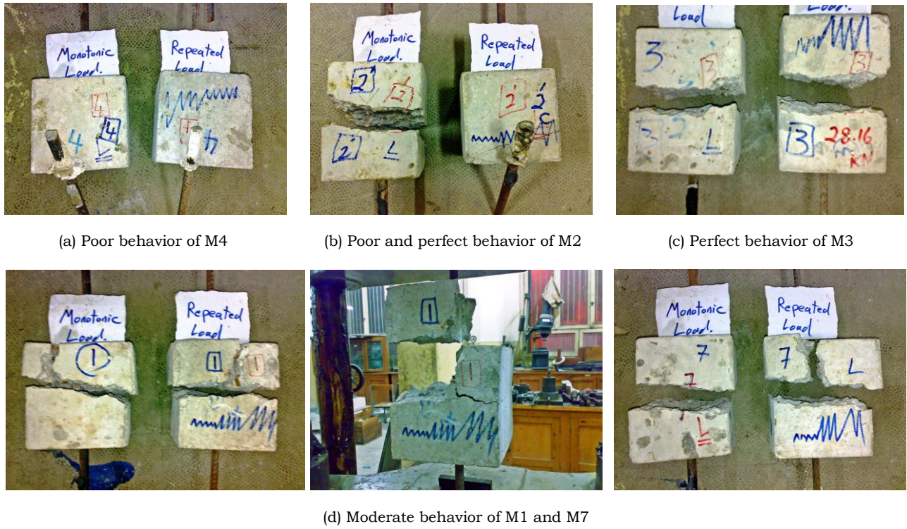
Fig. 22. Effect of cyclic loading on modes of failure.
