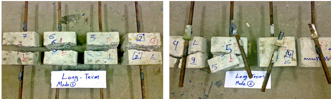
Fig. 19. The two extremes modes of failure at later ages under monotonic loadings.
