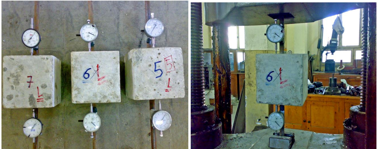
Fig. 3. Dial gages attached to the specimens.
