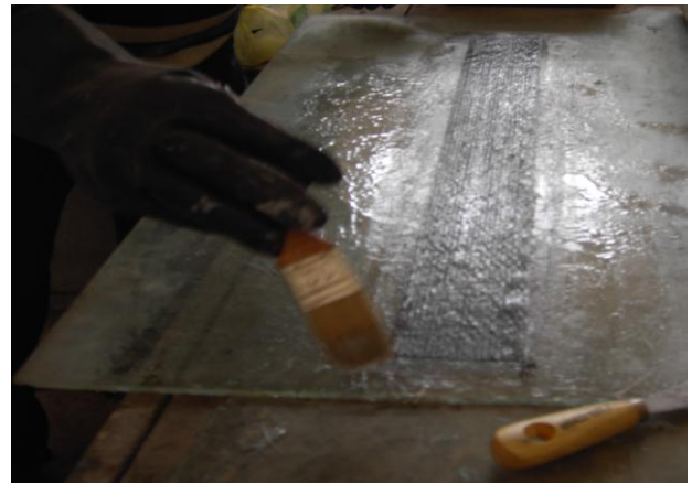
Fig. 6. Manufacturing intertwined rods from FRP wraps.
