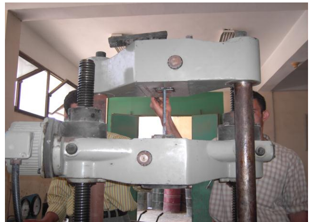
Fig. 7. Testing intertwined GFRP rods.
