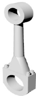
Fig. 10. Designed connecting rod.
