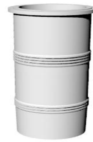
Fig. 9. 3D model of cylinder liner.
