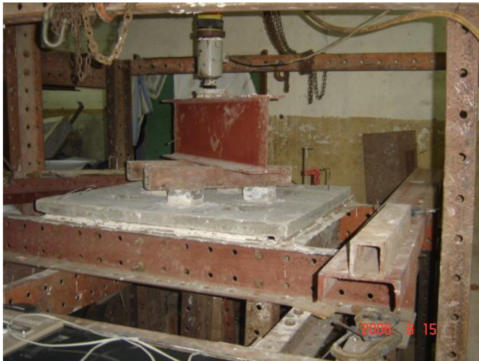
Fig. 4. One of the tested slabs under load.
