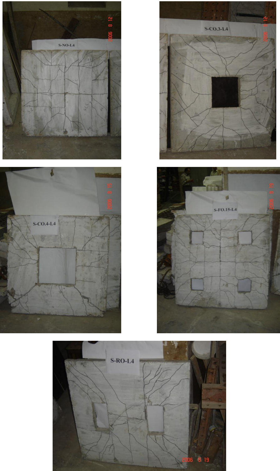
Fig. 15. Cracking patterns of slabs tested under four loads after failure.
