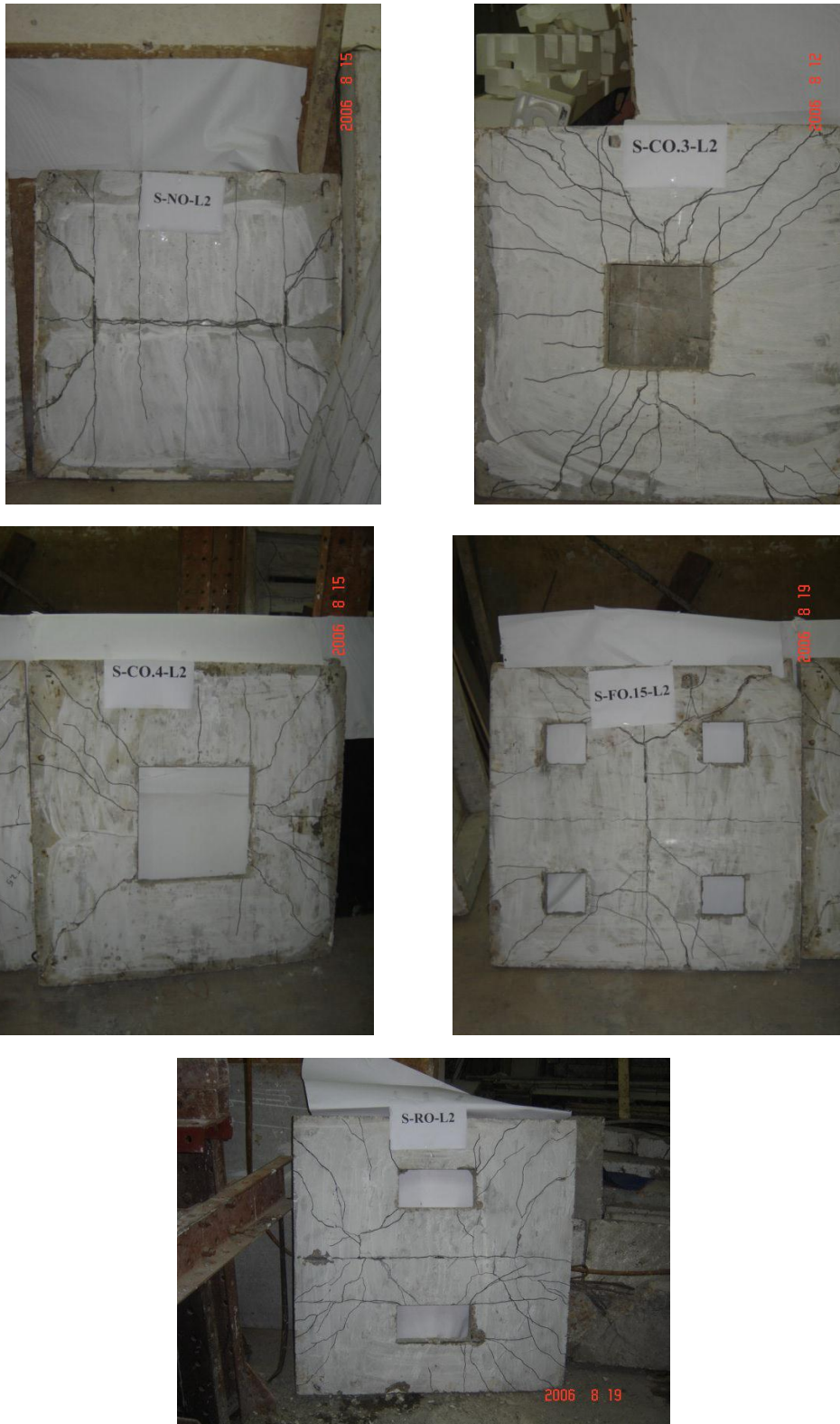
Fig. 16. Cracking patterns of slabs tested under two loads after failure.
