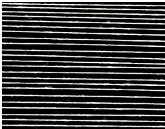
Fig. 3. Appearance of slub yarn (Ne 10, twist factor 4, pressure 3 bar and pulse duration 0.08 sec)
