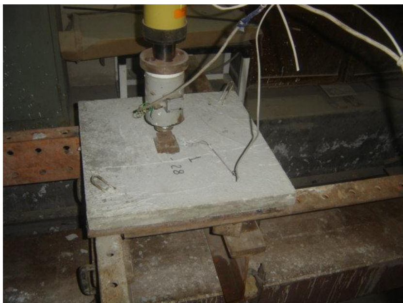
Fig. 2. One of the tested reinforced concrete slabs under load.
