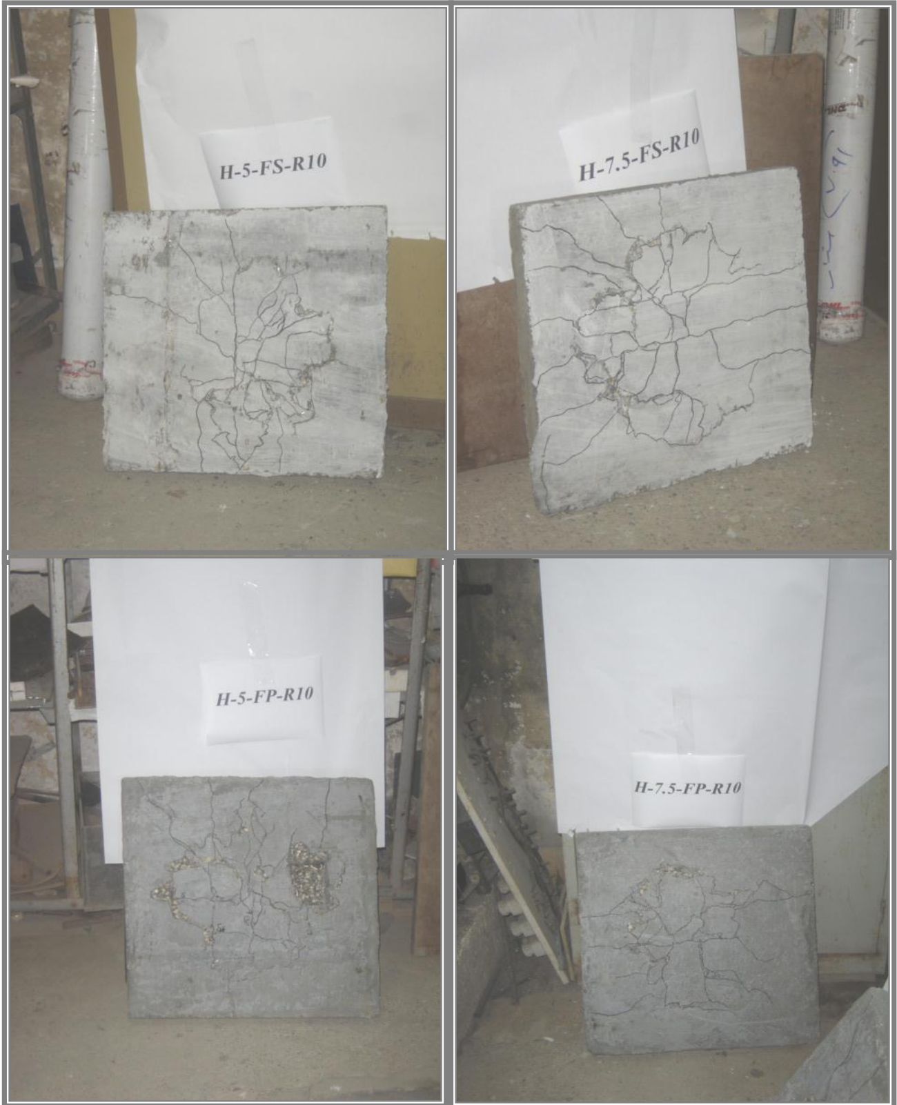
Fig. 13. Cracking patterns for tested high strength concrete slabs with fibers.
