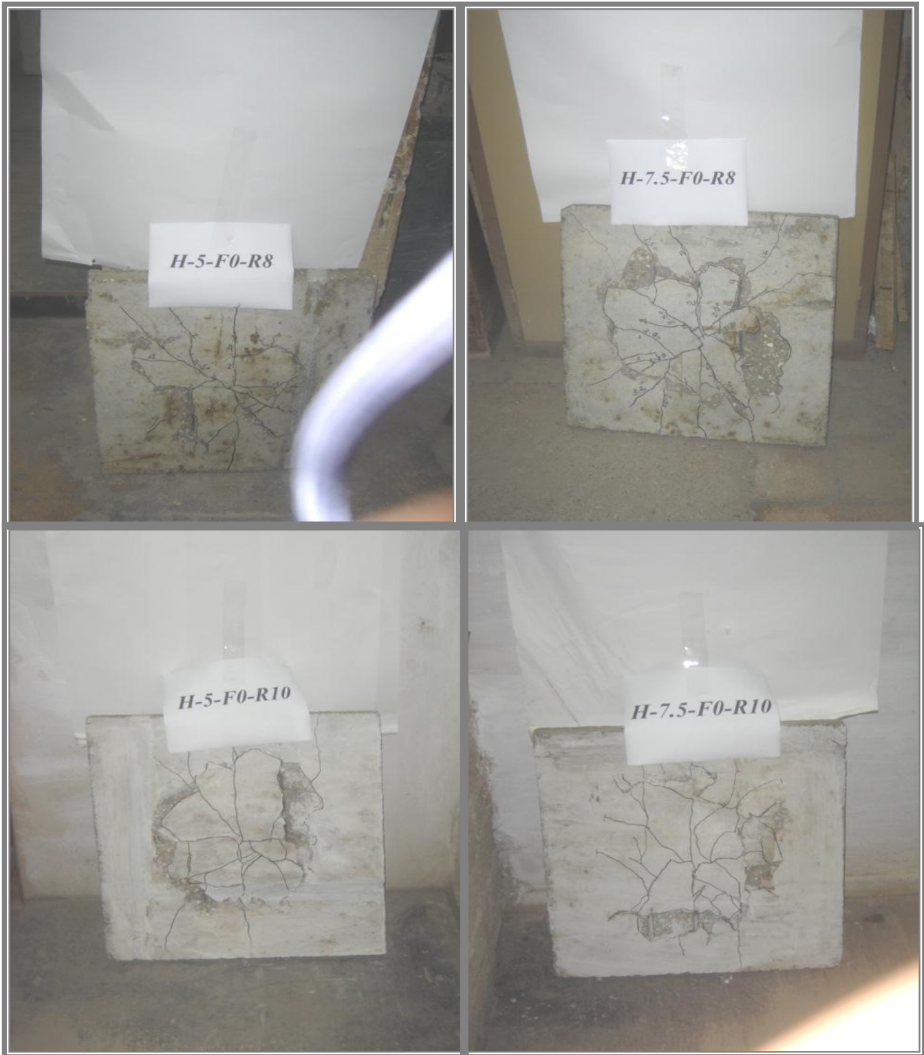
Fig. 12. Cracking patterns for tested high strength concrete slabs without fibers.
