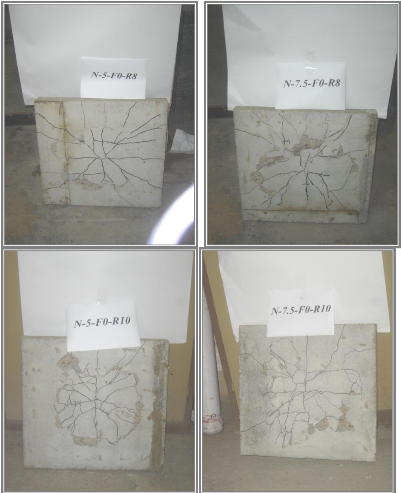
Fig. 10. Cracking patterns for tested normal strength concrete slabs without fibers.
