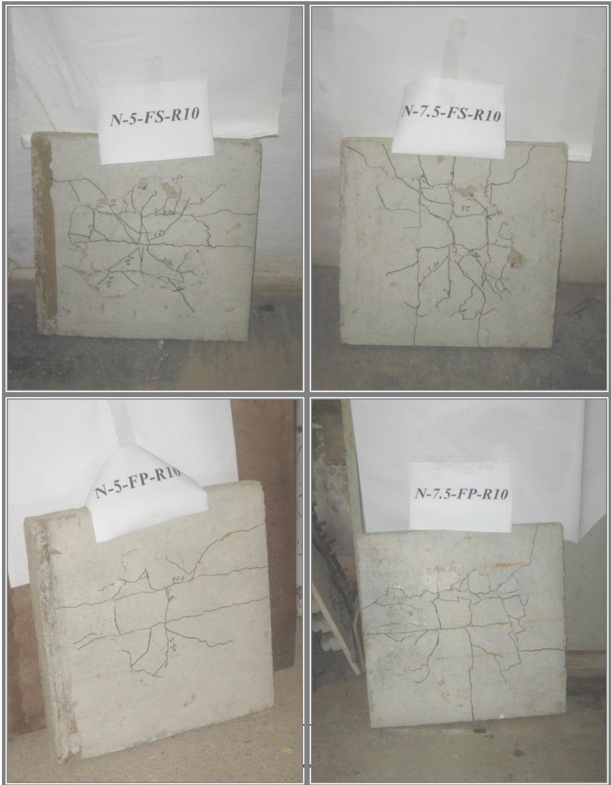
Fig. 11. Cracking patterns for tested normal strength concrete slabs with fibers.
