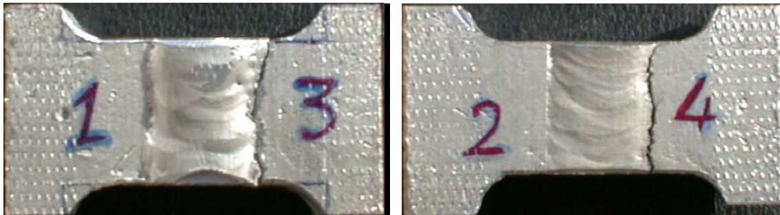
Fig. 12 Example for fractured specimens after tensile testing.
