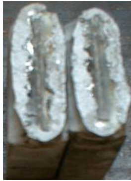
Fig. 4. Failed specimen no. 4 which fractured after second pass.
