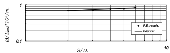
Fig. 15. Lateral Displacement ratio, (\Delta/L)_{mS} versus Pile Spacing ratio, S/D . ( D=0.60 m, L/D=30 , T_a/D=3 , B_a/D=2 , E_p/E_s=500 , \phi=30^\circ , P_h=300 kN/m).
