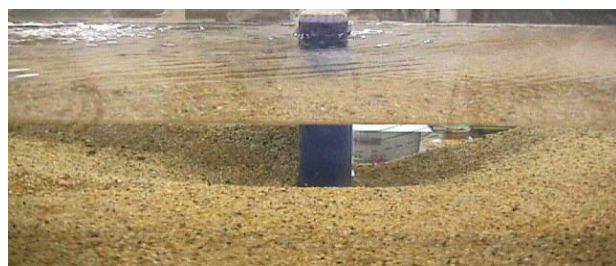
Fig. 3. View of final phase of scour hole around dike.
