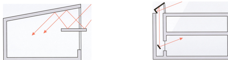
Fig. 10. Passive light-shelf (left) and light- pipe (right) designs can introduce adequate ambient daylight for office tasks in a 4.6 m to 9.1 m zone of a deep perimeter space [20].
