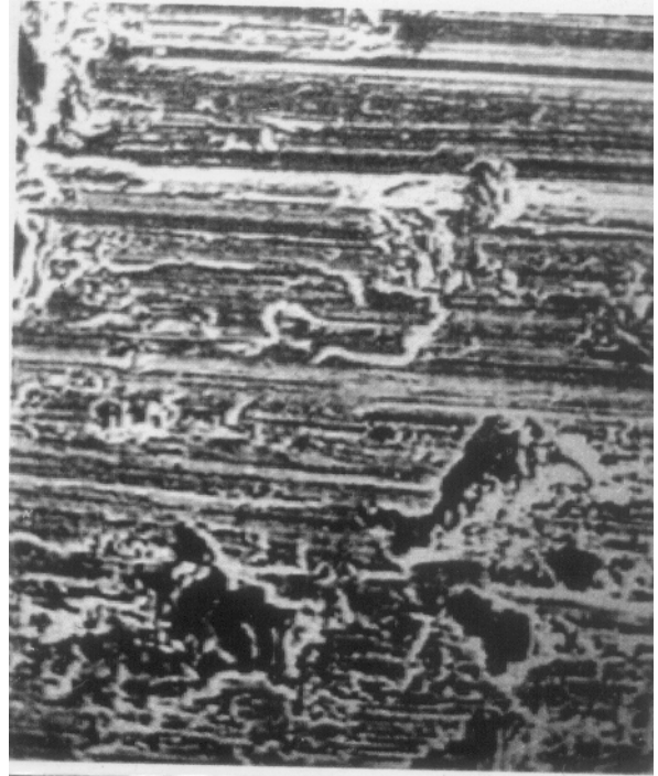
Fig. 14-b. Micrograph of worn surface of composite squeeze specimen at 150 °C X-250.
