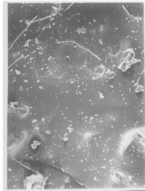
Fig. 15-a. Micrograph of worn surface of composite vortex specimen at 250 °C X-250.
