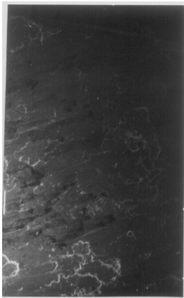
Fig. 13-b. Worn surface of the steel disk against sliding of 8 vol. % squeezed composite specimen X-250.
