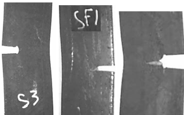
d) S3 at ultimate load e) SF1 with crack initiation f) S3 loaded beyond ultimate load
