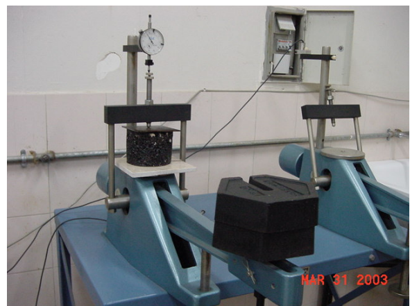
Fig. 4. Specimen under static creep test procedure.
