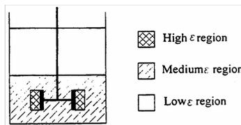
Fig. 5. Batch mixer (agitated tank).
