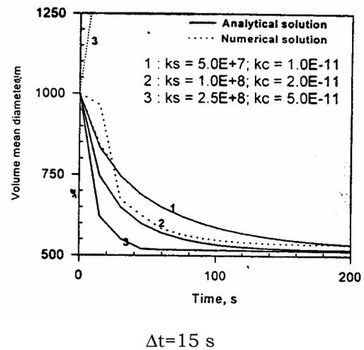
Fig. 9. Effect of breakup coefficient on numerical solution.
