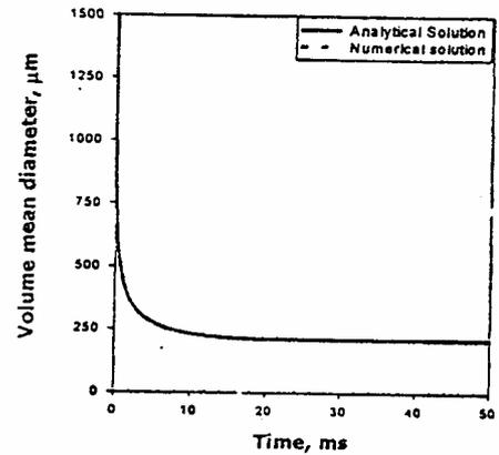
Fig. 17. Comparison between adaptive numerical solution and analytical one for high breakage rate.
