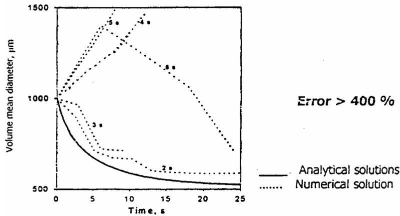
Fig. 4. Effect of fixed time interval on numerical solution.
