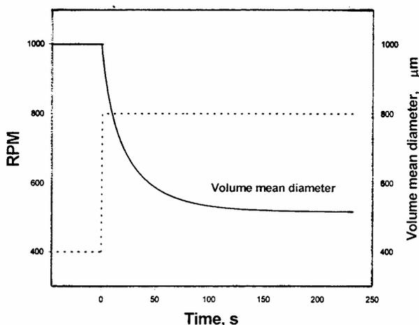
Fig. 6. Effect of RPM on volume mean diameter.
