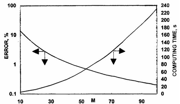
Fig. 14. Effect of M on error and computing time.
