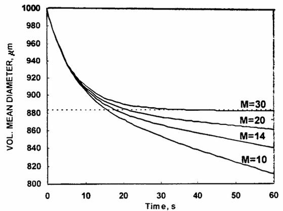
Fig. 13. Effect of M on quasi-equilibrium drop size (net breakage).
