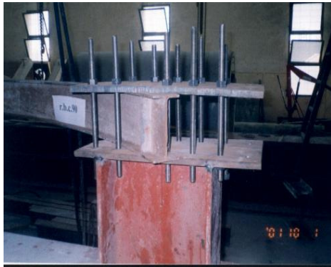
Photo 1. Typical support for tested beams.
