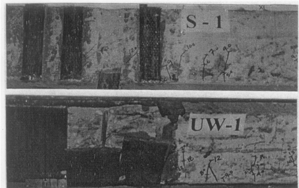
Fig. 6. Cracking patterns for strengthened beams (S-1) and (UW-1).
