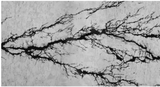
a- River branching cracks.
