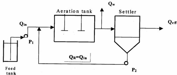
Fig. 1. Activated sludge pilot plant.
