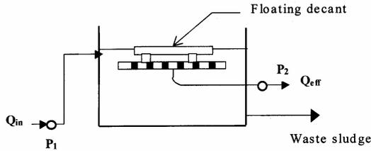
Fig. 2-a. Sequencing batch reactor (SBR) pilot plant.
