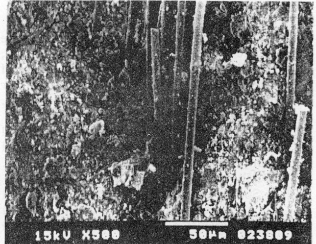
Fig. 10. SEM micrograph of fractured surface for 0.4% carbon fiber reinforced concrete.
