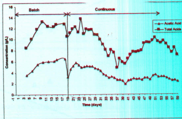
Fig. 2. Product acid concentrations for bagasse/chicken manure fermentation B.
