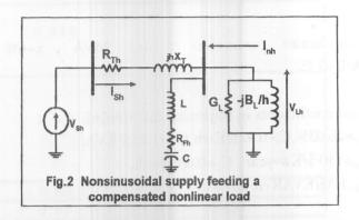
$$\overline{I_{sh}} = \frac{\overline{V_{sh}} \ \overline{Y}}{1 + \overline{Z_{Th}} \ \overline{Y}} - \frac{\overline{I_{nh}} R_{Fh}}{R_{Fh} + \overline{Z_{Th}}}.....(18)$$
