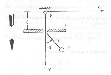
Consider a bob of mass "m" moving in the vertical (x,y) plane, at the end of a light taut chord of fixed length  $r_o$ . The chord passes through a slot in moving board whose motion is constrained in a vertical straight line and the other end of the chord is fixed at O, Denoting  $\xi(t)$  as the vertical displacement of the board at any instant t and setting Oxy as a fixed frame of reference one can write the coordinates of the bob as
