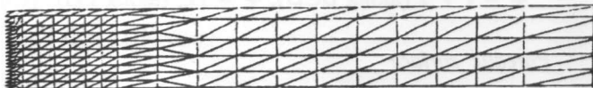
Figure 2. A finite element mesh for a partilly penetrating well No. of elements = 405. No. of nodes = 238.
